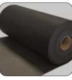
Cross-linked Polyethylene Foams are produced by admixing selected amount of chemi cal cross-linking agents and chemical foaming agents in an extruder and conveying the resultant hard plastic polyethylene panel through an oven. Thanks to its production technology, the XLPE foams produced with closed porosity and smooth surface have superior mechanical and thermal properties due to the cross-linking in their structure.
